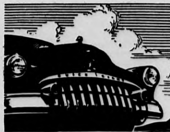
FOUR-WAY FOREFRONT. This rugged front end (1) sets the style note, (2) saves on repair costs—vertical bars are individually replaceable, (3) avoids "locking horns," (4) makes parking and garaging easier.
