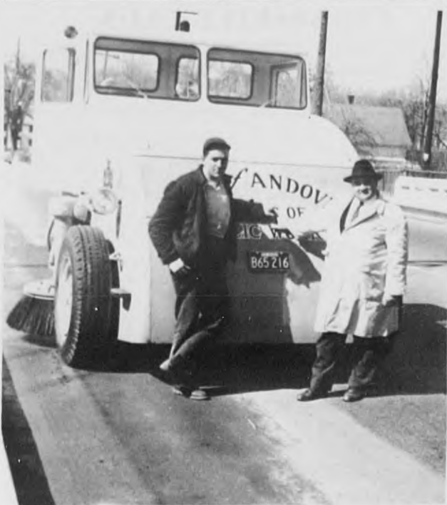
OPERATION CLEAN SWEEP - The town's new street sweeper, with a four cubic yard capacity, has hydraulic controls to lower and raise the brushes. Highway Supt. Stanley Chlebowski, right, and operator Bill Douty, left, posed in front of the machine Monday, as it made a trial run along North Main st. The sweeper is getting immediate use, as the annual clean-up campaign gets underway to rid the town of the winter's accumulation of sand. (Staff Photo)
